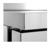
Sharp-edged worktop Reinforced worktop with sharpedged front edge, splashback h 100 mm with 10 mm inner radius and rear closure to avoid dirt accumulation.
